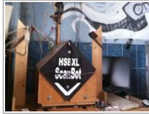
A scanner for books made from the remains of cleaning machine, (cameras, scanners glass (IRIN
